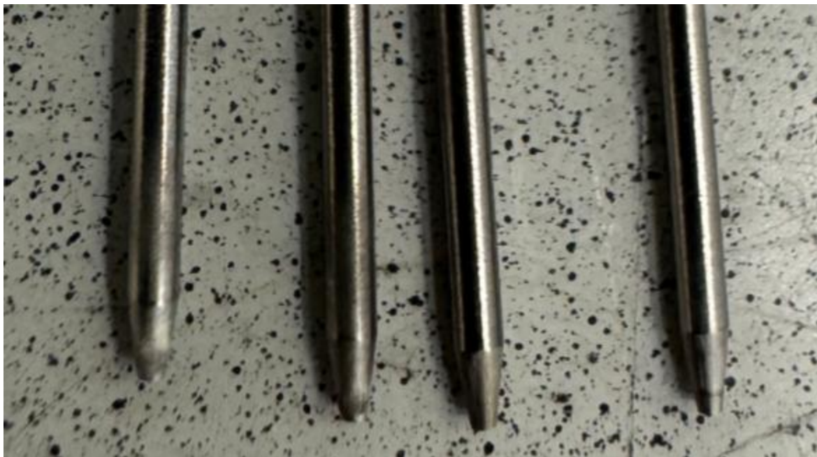
Figure 5: degradation of tungsten electrode, type WS2 (1mm with top angle 18° & top diameter 0,5mm): 2 left are used electrodes and the 2 right are new ones
